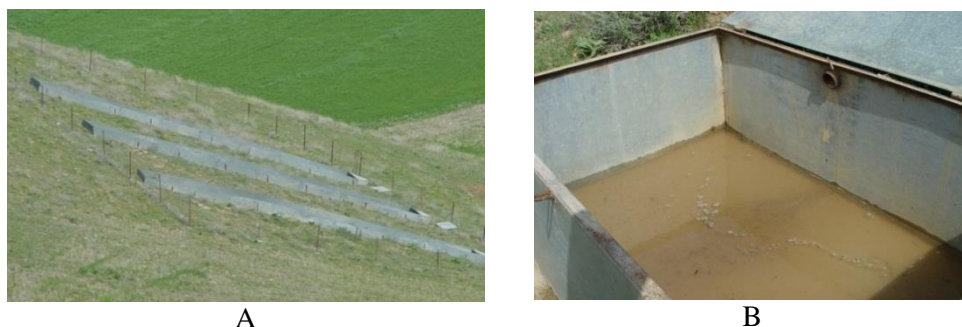
Fig. 3. A view of standard erosion plots (A) and a view of runoff and sediment collected in plot output reservoir (B).
