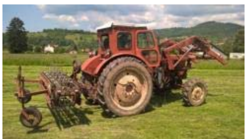
Picture 1 chain finger side delivery rake
